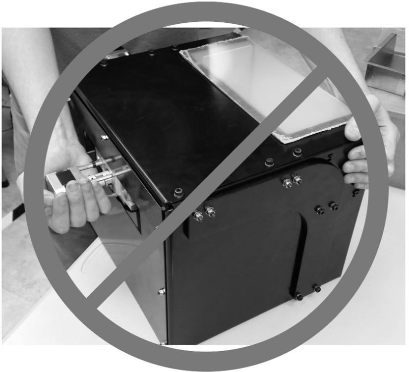
Place Ghost Gunner on a smooth surface in a shop environment conducive to stray aluminum chips. Ghost Gunner must operate in the upright position to prevent chip ingress to sensitive linear components.
